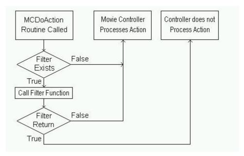
Figure 15. Using an Action Filter Function
