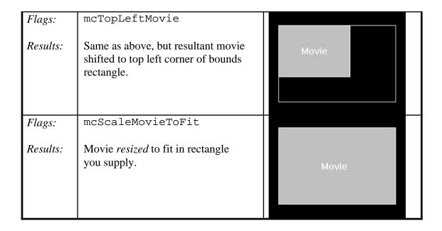
**Attached Controllers:** Calling MCPositionController on an attached controller requires specifying only one rectangle for both the movie and the controller (the second rectangle is ignored and should be coded as NULL). The way the rectangle is used depends on the flags you provide:
