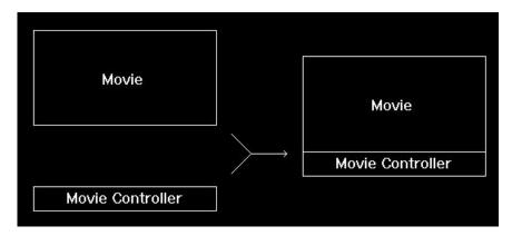
Figure 12. How SetControllerAttached works.
